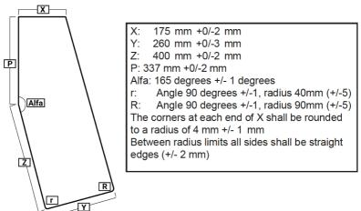
3.4.2.2 The thickness of the rudder (excluding bevels) shall be not less than 14 mm (12 mm for wooden construction) and not more than 15 mm. Bevelling is permitted between the edges and the bevelling limits, situated 60 mm from all edges. No bevelling is permitted on the top of the rudder head.
