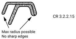
3.2.2.16 GRP Hulls. For wood and wood/epoxy hulls, see plans
