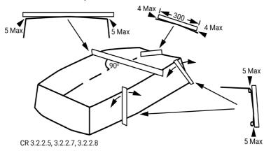
On GRP hulls only, for the purpose of this and other 'panel flatness measurements' the extent of the panels will be limited by an edge zone, defined by the 'Standardized Edge-Edge-Zone Finder'.
